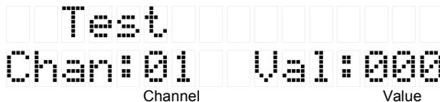
Pressing <◀> and <▶> buttons select channel, and <▲> and <▼> buttons to change his value. The ìAllî keyword allows you to control all channels at one time. <Enter> and <Menu> buttons end test mode.
